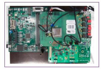
Figure. 2. PCB view of the prototype arbitrary waveform generator. DAC manufacturer demo board was used for the current prototype.
