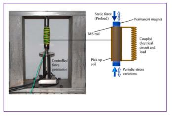
Figure 1. Generator scheme. A rod of MS material is inserted in a pickup coil, this latter connected to an electric impedance. Two permanent magnets provide the magnetic bias. The material is preloaded with a constant stress, while a time varying mechanical load is exerted longitudinally along the rod axis.
